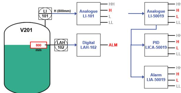
Consider also when multiple alarms are generated by the same point. In the real example at the right-hand side of the picture, high and low alarms were generated at the same setting on the analogue input block, the PID control block and an alarm block. Triplicate alarms!
